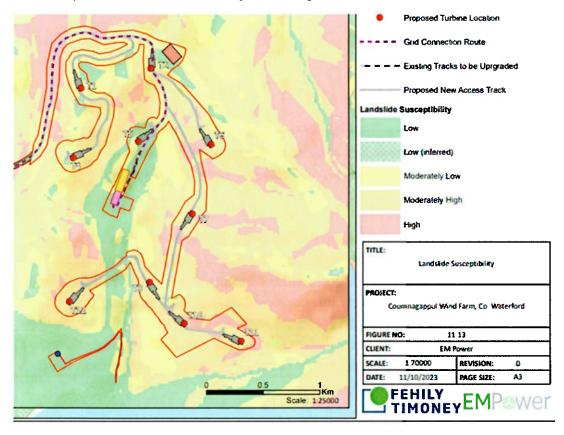
As can be seen on the map above, turbines are located on areas rated "moderately high" and "high" on the landslide susceptibility map.
